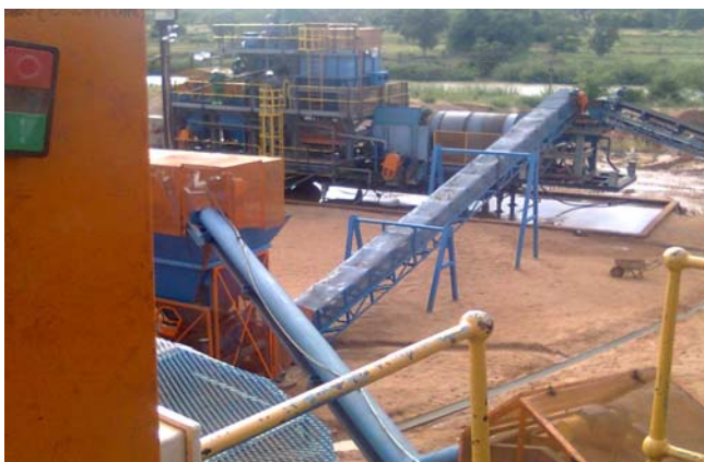
The Density Medium Separator
